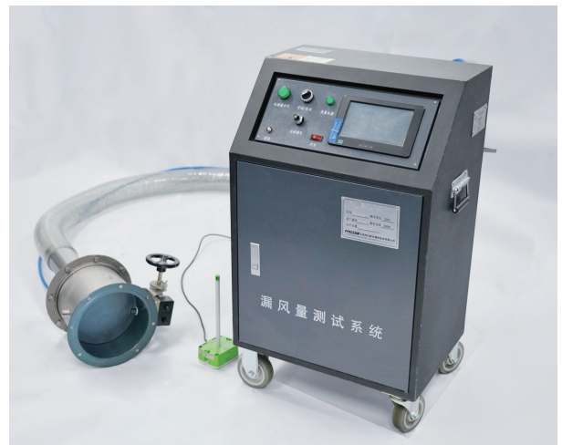
Damper Air Leakage Testing Facility
