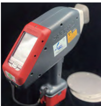
PMI Spectrometer For Stainless Steel Material Inspection
